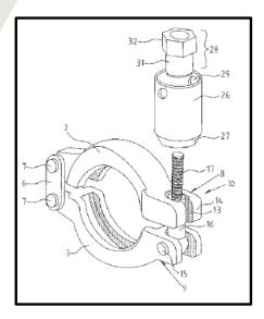
The patented safety clamp design has been in use for almost two decades. It has proven to be indispensable for the safety conscious engineers and managers globally. The design enables the leak before-burst scenario that is at the heart of ASME BPVC codes and standards.
