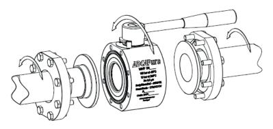
Loose body flanges make it possible to install the valve without aligning of the welded end connections. After installation the valve can rotate on 360° for the desired orientation.
