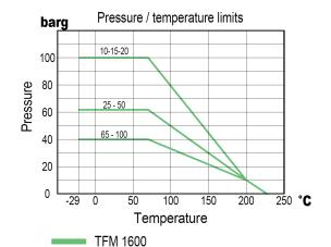
Note: Working pressure may be limited by the valve connections.
