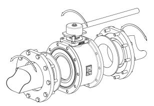
Loose body flanges make it possible to install the valve without aligning of the welded end connections. After installation the valve can rotate on 360° for the desired orientation.
