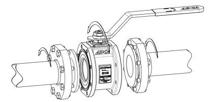
Loose body flanges make it possible to install the valve without aligning of the welded end connections. After installation the valve can rotate on 360° for the desired orientation.
