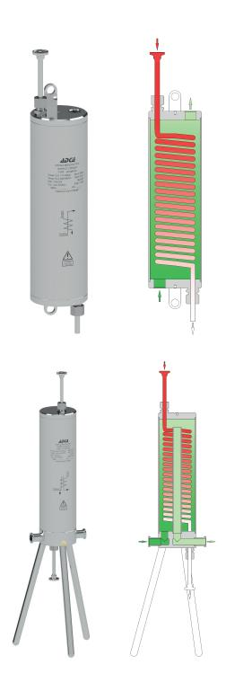
PERFORMANCE: 30 to 60 kg/h of sample water at  $\approx$  30 °C with 1 m<sup>3</sup>/h - 15 °C inlet cooling water (boilers up to 20 bar - 220 °C). For other pressures, temperatures and/or certified values, consult manufacturer.
