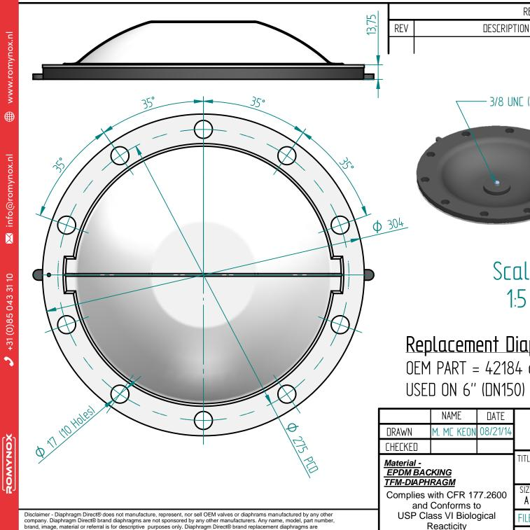
guaranteed to fit OEM equipment and meet or exceed OEM specifications. Diaphragm Direct® brand replacement diaphragms are
