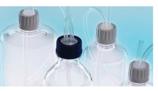
Liveo<sup>™</sup> Pharma Bottle Closures include a one-piece silicone stopper made from biomedical-grade platinum-cured silicone elastomer molded with high-purity platinum-cured silicone tubing. This makes Liveo™ Pharma Bottle Closures particularly suitable to seal threaded glass and plastic bottles and containers used for critical high-purity fluids and media in biological drug production.
