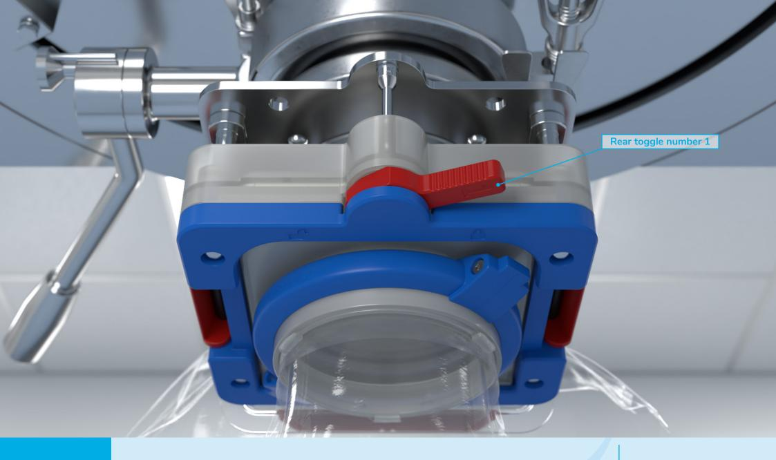
Fully turn the rear red toggle, marked number 1, to lock the chargebag in place and release the active & passive interlocks.
