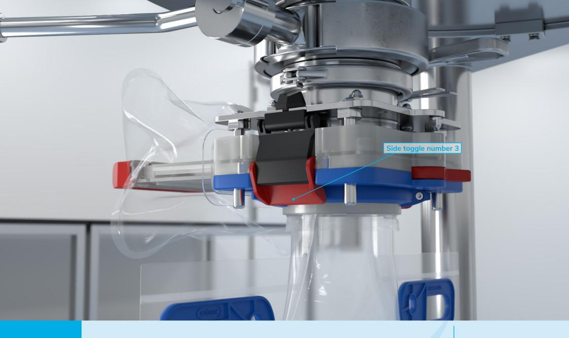
At this point there is a void in the system, and so the two red side toggles, marked number 3, need to be fully lowered. This raises the active cassette onto the active spigot and creates a contained seal.
