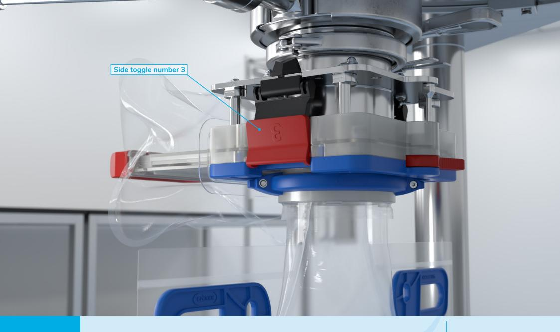
Having closed the isolation valve, the chargebag can be removed by reversing the docking procedure:
