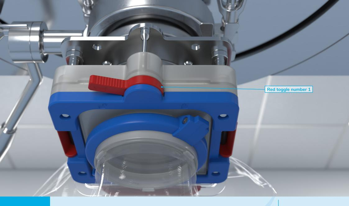
Finally fully turn the rear red toggle marked 1.
