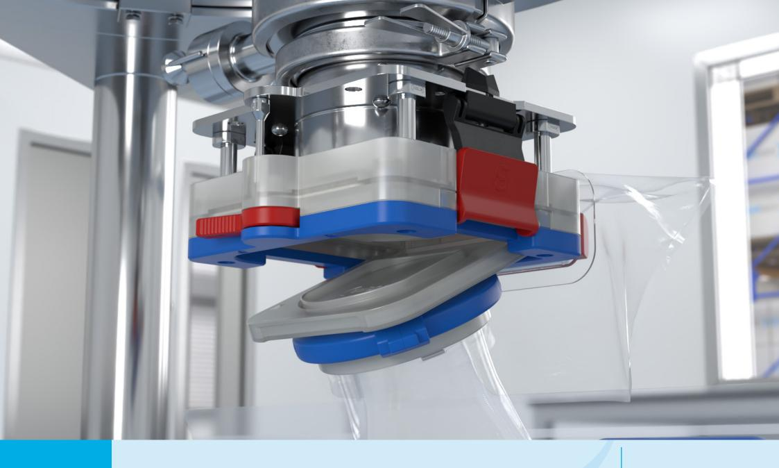
Dock the chargebag, by sliding the front of the passive under the lip of the CSV Active.
