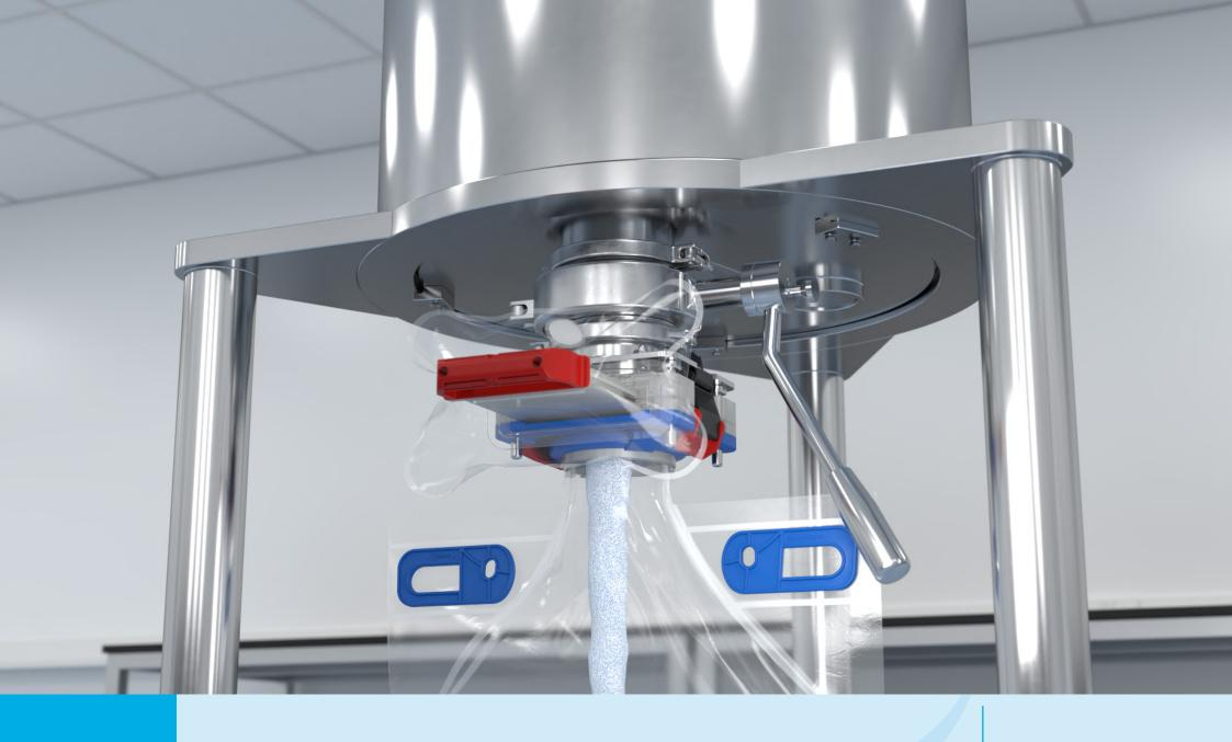
To fill the chargebag, open the isolation valve above the CSV Active and dose as required.
