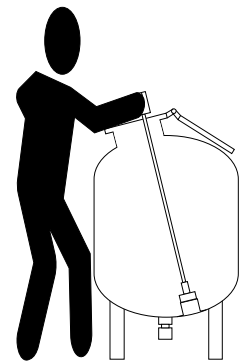
Picture 5: Installation with a multi tool when you can't reach the tank plate.
