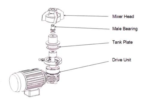
Picture 1. Equipment tested, schematic overview from the manual sent by the commissioner.
