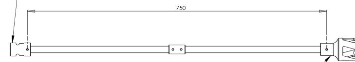
Default length for 20 and 30mm is 750mm, Extension step 750mm Default length for 12mm is 400mm with 400mm extension.
