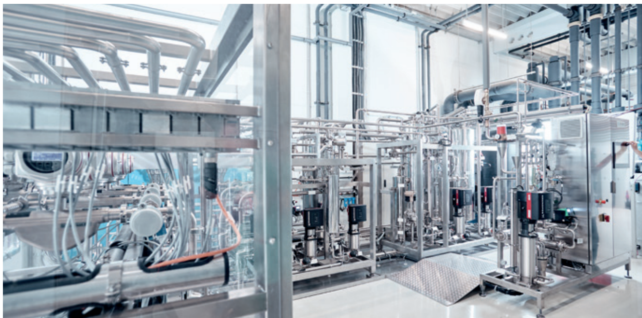
Process test bench. Cycle and lifetime testing of diaphragms and valves with saturated steam and various cip media.
