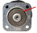
• Place the support spiral (from MD 65) back into the bonnet. The last winding of the support spiral (see right arrow) must not end on a compressor ridge.
