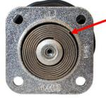
Place the support spiral back into the bonnet. The last winding of the support spiral (see right arrow) must not end on a compressor ridge.
