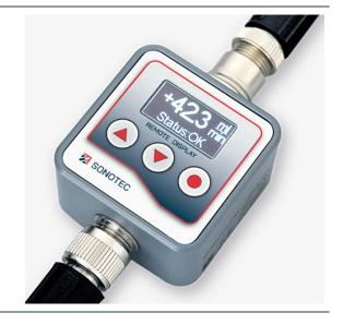
The Remote Display RD.10 enables real-time flow monitoring without a PC or PLC. The sensor accessory shows the current flow rate, the volume, the internal sensor temperature, the minimum or maximum flow as well as the measuring state. With plug-in connectors it can be easily connected to all SONOFLOW and SEMIFLOW CO.65 sensors.
