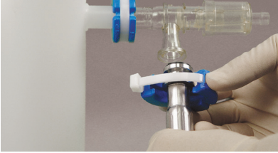
Position SaniSure Clamp around tri-clamp fitting
