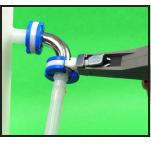
Tighten the cable tie by squeezing the trigger one or more pulls - The cable tie is automatically cut off flush when the tension setting is reached.
