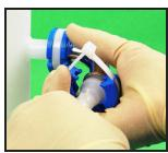
Position SaniSure Clamp around sanitary clamp fitting. Insert cable tie end and slide clamp closed.
