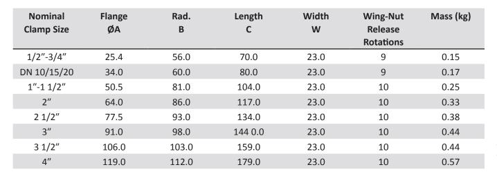
Wing-nut rotations are measured from the clamp starting in its optimum clamping position (segments parallel when assembled), to the safety eyebolt being able to swing free. One rotation = 360°
